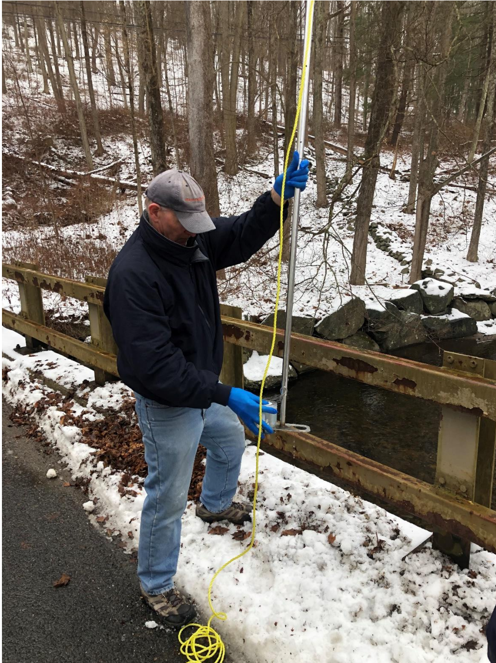
Bill Wright prepares to lower a Cyclopure cup off of the Silver Hill road bridge in Easton to collect water for PFAS analysis
